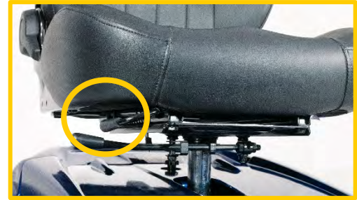
Figure 6 – Pull black handle to adjust the backrest
