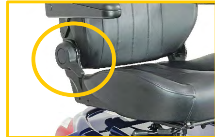
Figure 4 – Pull black handle to adjust the backrest
